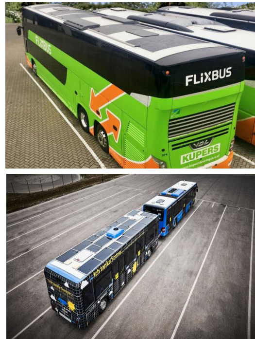
Figure 6.3. Flixbus diesel bus with PV modules on rooftop (top) Munich Transport Company's diesel bus with PV modules on the rooftop (bottom)
