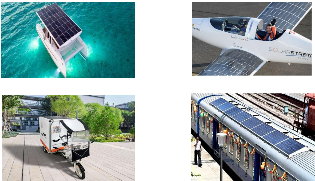
Figure 6.4. Boat with solar PV integrated (top left), Aircraft with integrated solar PV (top right) Cargo Bikes & Tuk Tuks (bottom left) Train with solar PV modules attached (bottom right)
