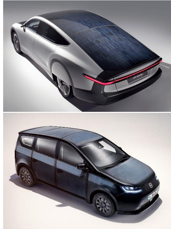
Figure 6.1. LEV with PV rooftop from Lightyear (top) LEV with PV rooftop and body from Sono (bottom)
